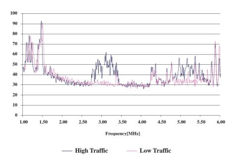
Measured spectrum (@approx 3m from powerline system) At high and low data traffic states: note reduction at low traffic state.
