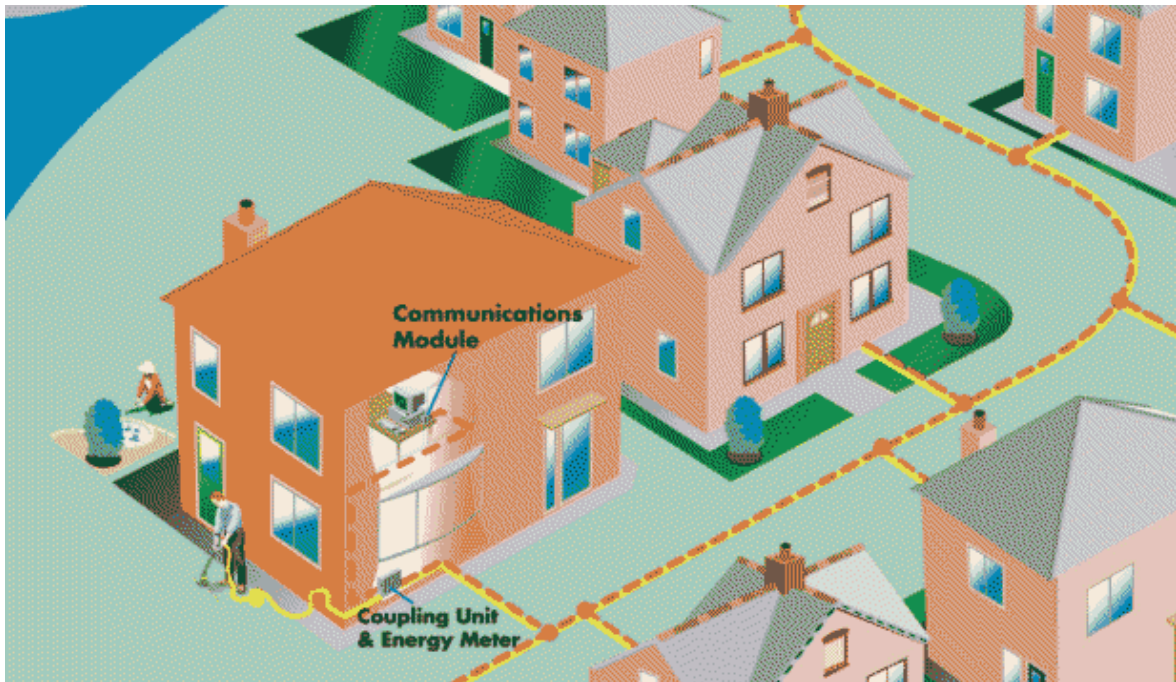
Figure 5: Last Mile PLC (Source: NOR.WEB)
